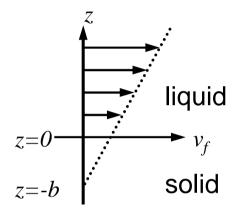
Slip length, *b*, models effective position of interface Negative *b*, effective interface moves to liquid side of boundary
